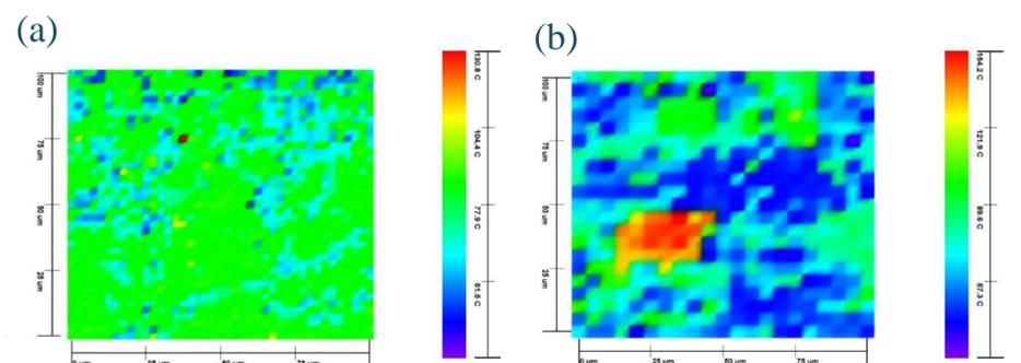
**Figure 3.** TTM maps of hot melt extrudates prepared at 150°C (a) and 110°C (b).
