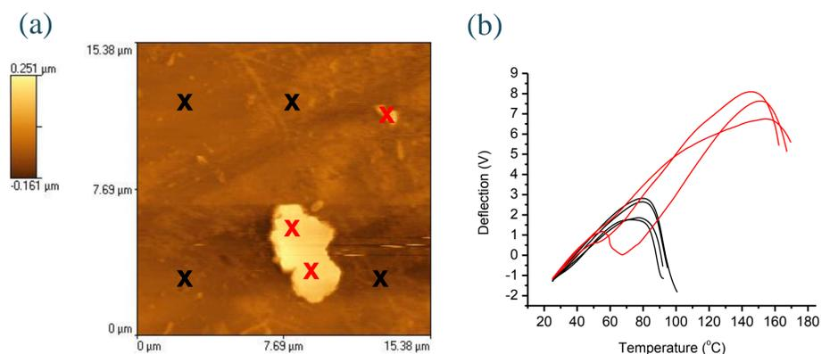
**Figure 2.** Topography image (a) and representative LTA scans (b) at locations marked with an x.
