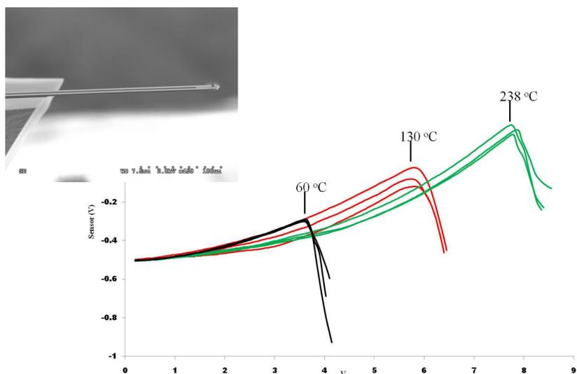
**Figure 1.** Local thermal analysis scans on three polymeric standards and a SEM micrograph (inset) of the probe used to carry out the measurements.
